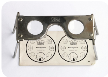
Figure 2. An old Zeiss pocket stereoscope with original test image.
