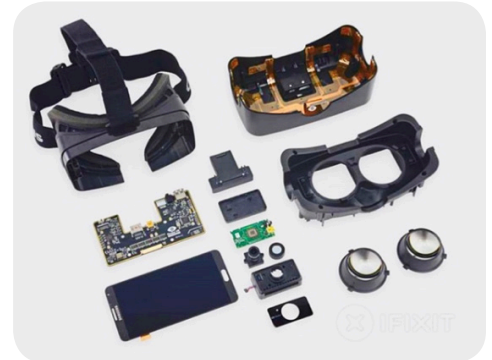
Figure 1. A deconstructed VR headset.
