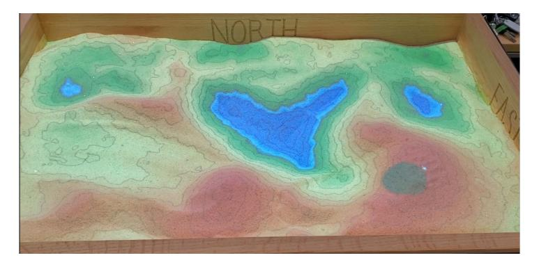
An AR Sandbox is a real sandbox that uses virtual topography (study of landforms and features) and water that is created with the help of a Microsoft Kinect 3D Camera, a projector, and some software from the computer. Using this technology, we can move the sand around in the sandbox and learn about geographic concepts in real time! However, since there are many of you and only one sandbox, we need to go over some rules!
