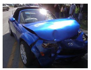
to limit the deformation to the car's frame while keeping the passenger cabin intact. When combined with other safety features, like seatbelts and airbags, the likelihood of the occupants surviving in an automobile crash increases significantly. Although crash zones end up leaving more physical damage to the vehicle in a crash, the safety it provides far outweighs the cost to repair.
