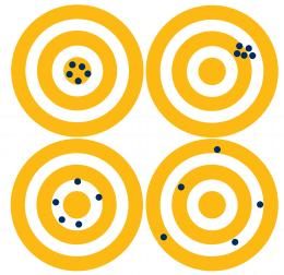
characteristics. Tolerances provide acceptable boundaries that account for minor imperfections. High accuracy ensures that parts are consistently produced near the target dimension, and tight tolerances demand precise control of the manufacturing process to ensure that any deviations remain small and within the allowable range.
