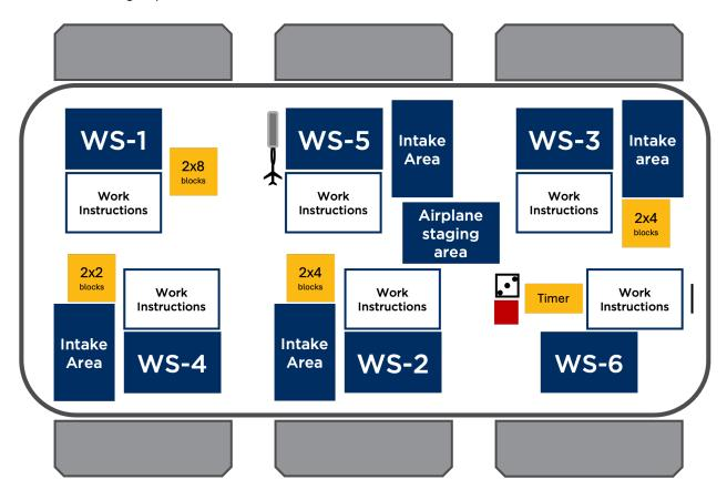
Since Phase-1 simulates the traditional facility, one whose layout has been designed around departments or over time growth, production should be as difficult and cumbersome as possible. Additional obstacles may be placed in the room (size permitting) to further inhibit the workers' efficiency.
